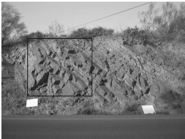
Figure 2. Rock exposure with well-developed discontinuity sets along a secondary road in Spain, from the towns of Falset to Bellmunt in Baix-Camp, Catalonia. The rock mass consist of Carboniferous Meta-Siltstone and Slates. According to BS: 5930:1999 the rock mass can be described as: dark-grey to black, silt-clay size, small tabular, slightly weathered META-SILTSTONES and SLATES. The dimensions of the white boards are 60x60 cm. The size of the outlined area that is used for the laser scan analysis is 4x4 meters (see Figures 3 to 5).
