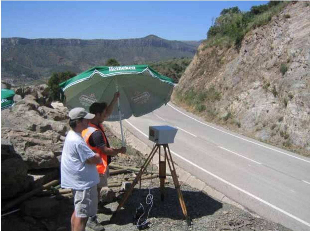
**FIGURE 1. Typical field set-up of a laser scanner (Optech 3D Ilris scanner [30]) . The umbrella is to keep the scanner cool and to be able to read the display. Persons in picture: John Kemeny (left) and Bart van Knapen (right). Location: Along road T710 between Toroja and Vilella Baixa, Priorat district, Catalan Province, Spain.**
