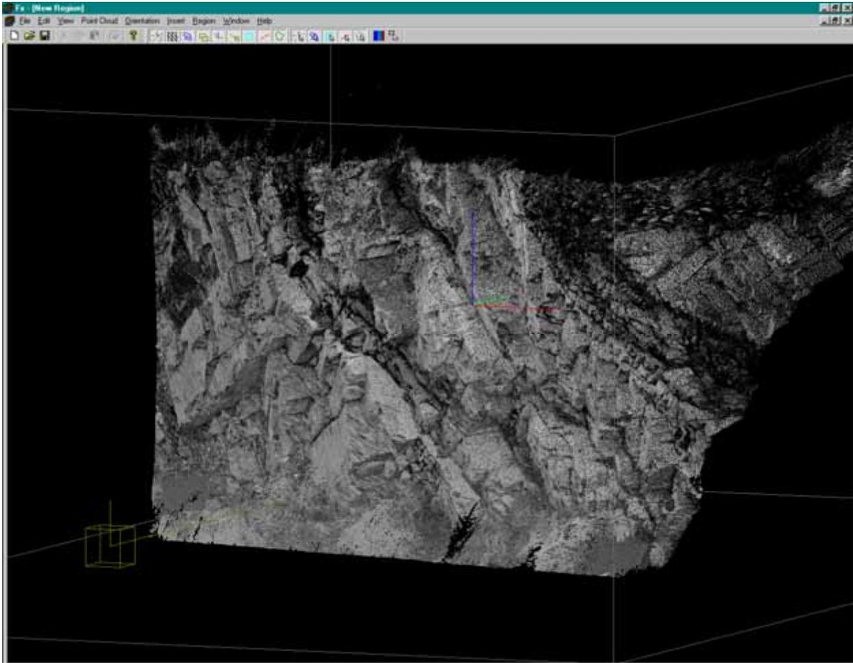
**FIGURE 3. 3D visualization of the entire point cloud (with the software Fx, beta version 1.0 from Split Engineering [29]) of the scan made of the slope in FIGURE 2. The reflected laser intensities are shown in greyscale (i.e. white is high reflection and black is low reflection).**
