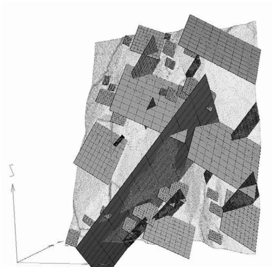
**FIGURE 7.** The figure here shows the individual discontinuity planes of sets 2 (dark-grey, semi-vertical planes) and set 3 (the bedding planes), modeled as linear trend surfaces. By calculating the distances between the individual surfaces, joint set spacing can be computed.
