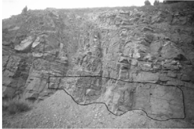
Figure 4. Photo of the scanned rock face, the area for which the orientation analysis (Figure 6) is done has been outlined.
