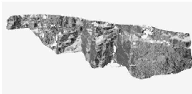
Figure 5. Digitally rendered 3D TIN of the selected rock section as outlined in Figure 4.
