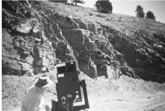
Figure 1. Cyrax 3D laser scanner in front of the surveyed rock face.
