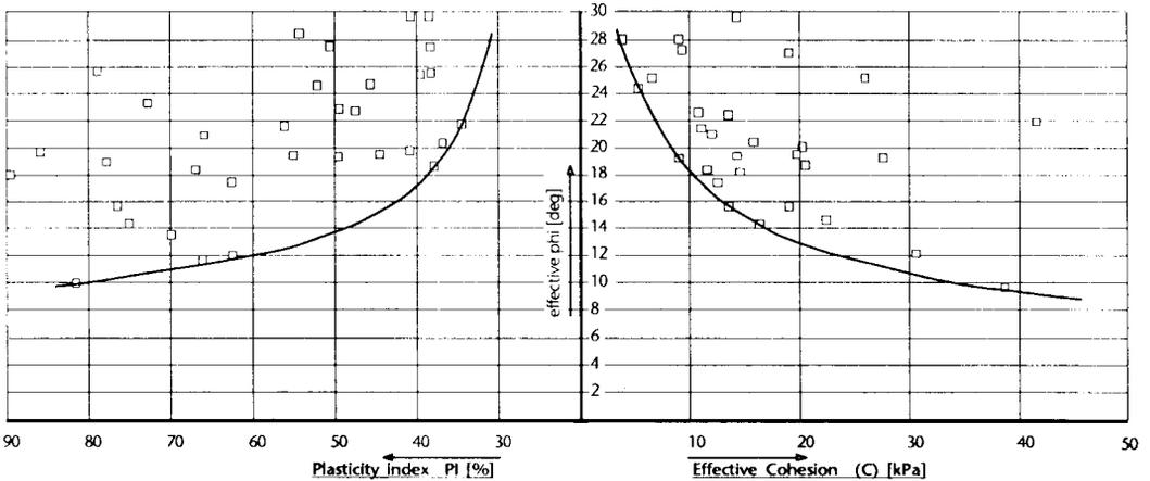
**Figure 2.** Examples Plasticity Index - effective phi and cohesion relation. (ch.7.4-4)
